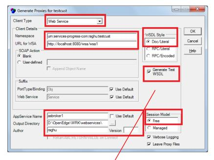
The job ProxyGen is creating the descriptor files the Web server will use to route a request to the right AppServer and the right ABL procedure. OpenEdge® Explorer reads the **Web Service**Mapping file that is part of what ProxyGen created, and uses this to deploy the procedure as a service.
