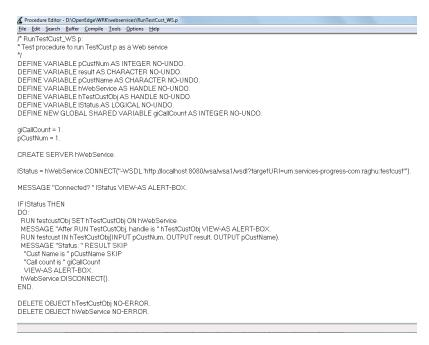
10. Run the above procedure. The output demonstrates that the web services *testcust* has been successfully consumed.
